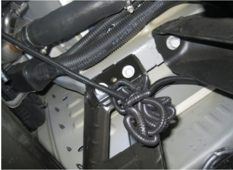
Figure 24. Excess wiring harness zip tied near the bed pass through grommet.
