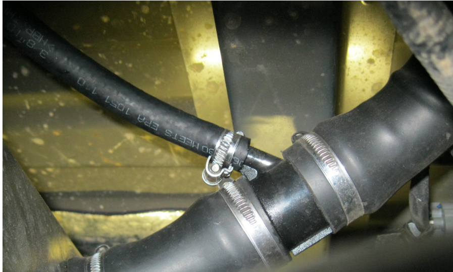
Figure 13. Transfer Flow fuel tee installed in the main fuel filler hose.
