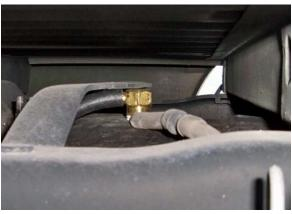
(Fig. 6) **NOTE:** Be sure that vent breather hose on rollover-stop vent valve, on the rear of the tank, is routed *under* the adjacent frame cross member as shown above.
