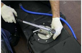
(Fig. 1) Loosen the hold-down ring on the OEM tank by turning counter-clockwise. Note where the connections on your vehicle's sending unit are "clocked" and install so they are located in the same position in the new tank.
