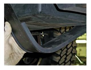
(Fig. 5) If optional TITAN Shield is not to be installed, install rubber bushings (pn 99 0000 0103) on both straps with the channel side toward the strap.
