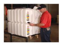
Step 8: Install poly union(s) into stand elbow kit(s).
