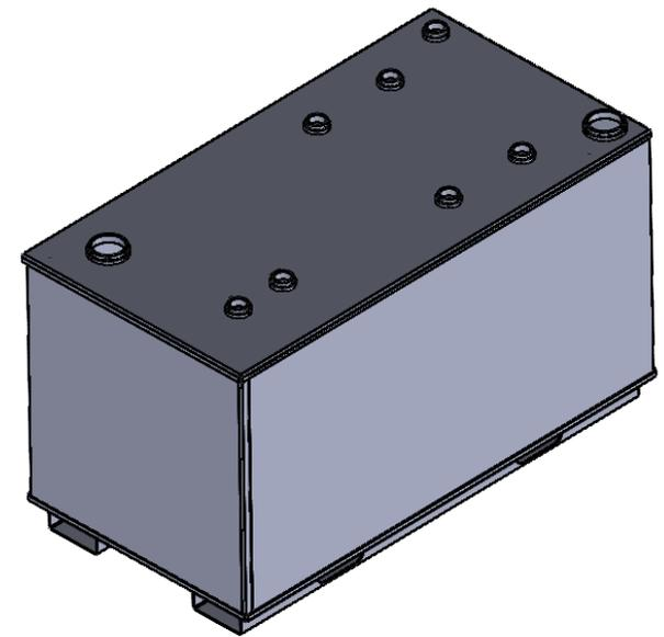
Any of the 2" Inner tank ports can be used for the Fill Cap, Pump, or Level Gauge.
