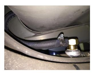
13) Place a washer on the  $\frac{1}{2}$  x 2  $\frac{1}{2}$ " bolts. Insert the bolts into the holes. Underneath the bed place a washer, spring, washer and then lock nut on the other side of the bolt. You will need two people to easily bolt the tank. Stop tightening the bolt once the spring starts to compress.
