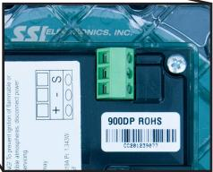
Auxilliary power and pulser connection at meter. Note three connections: DC+, DC-, and Pulser Signal.
