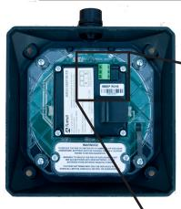
Three wire cable coming into the meter should be limited to only as much as is necessary to complete the wiring. Excess wiring should not be left inside the meter.
