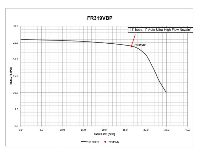
Changes in temperatures, fluid viscosity, and system accessories may shift the performance curves.
