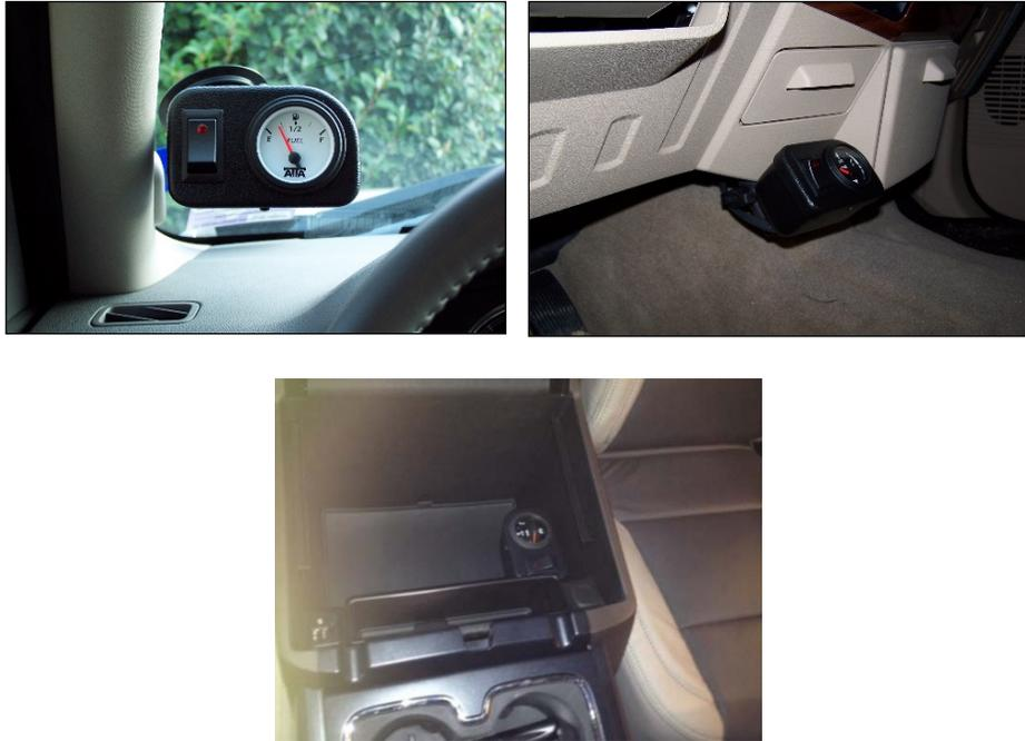
2. Place the Freedom Fill Controller Box under the instrument panel, (It may be necessary to remove the dash panel). This can be done by using two zip-ties to attach the controller to a factory harness or bracket. Insert the Controller harness to the Controller Box.
