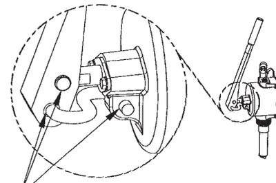
Lubricate all Pin Joints with grease to extend the life of your hand pump.
