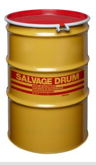
A Skolnik Open Head Salvage Drum is constructed of high quality carbon steel and meets the UN design type requirements. Standard Salvage Drums feature yellow bodies with yellow or red covers, with a multilingual salvage drum logo in red. Available options include 3/4" vent plugs and corrosion resistant epoxy phenolic lining. Each Skolnik Steel Salvage Drum tests successfully on relevant international standards, including the "T" rated salvage drum.
