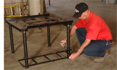
**Step 3:** Place drip tray insert pans w/screen into the drip tray holder spaces.
