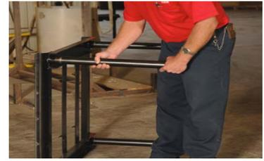
**Step 2:** Attach drip tray holder to front legs of stand. Leave ample space for your container below the drain valve.
