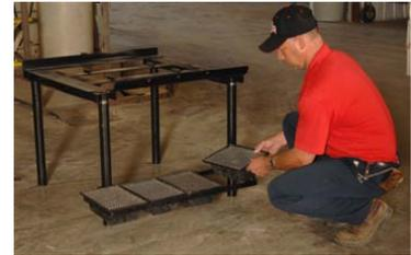
**Step 4:** Attach elbow kits(s) to front lip of the stand base, using 1/2" wrench. Repeat as necessary.
